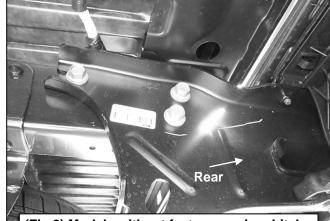
(Fig 2) Models without factory receiver hitch: Remove factory hex bolts attaching bracket to side of frame (driver/left side pictured)
